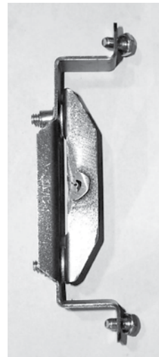
Latch Assembly re-assembled with Spacers removed.
