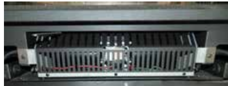
Secure fan with 2 screws removed in Step 1
